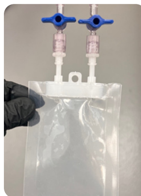
Figure 1: Image illustrating the test article PureFlex™ film bag with two ports.
