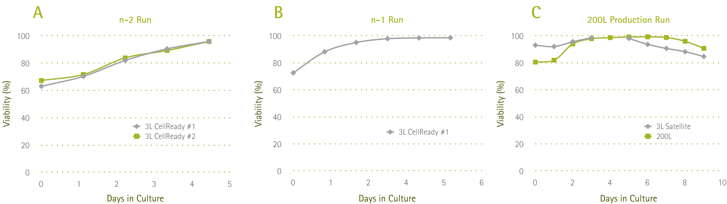
FIGURE 4: Viability (A) n-2 Run (B) n-1 Run and (C) 200 L Production Run. Bioreactors were run in batch mode, sampled daily and viability was determined using a Vi-CELL XR (Beckman Coulter). At each step, the cell viabilities remained consistently high. The low cell viabilities on day 1 of each run can be attributed to the presence of antifoam in the media, which is known to impair the measurement of viability.
