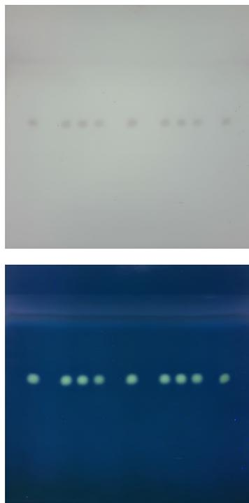
**Figure 5.** TLC Analysis of plate by the TLC Explorer under VIS excitation (top) and UV 366 nm excitation (bottom). The tracks 1, 5 and 9 are the references of dexamethasone acetate and 2-4 and 6-8 are the samples. The plates were derivatized with a mixture of dihydroxybenzaldehyde, glacial acetic acid and sulfuric acid.
