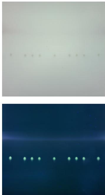
**Figure 6.** TLC Analysis of plate by the TLC Explorer under VIS excitation (top) and UV 366 nm excitation (bottom). The tracks 1, 5 and 9 are the dexamethasone sodium phosphate, reference and 2-4 and 6-8 are the samples. The plates were derivatized with a mixture of dihydroxybenzaldehyde, glacial acetic acid, and sulfuric acid.
