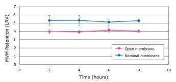
**Figure 3** One lot each of open and nominal membrane were used to evaluate MVM retention to an extended processing time of 8 hours.
