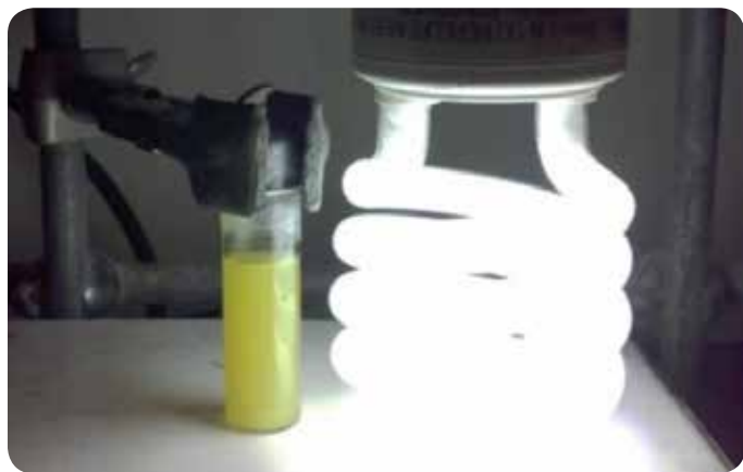
Figure 3. Photoreactor Setup With a 26 W CFL Lamp
