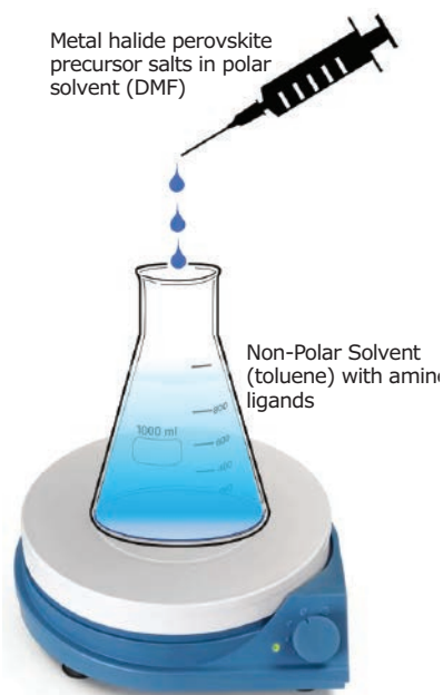
Figure 3. Schematic diagram showing the ligand-assisted re-precipitation (LARP) method. Reprinted with permission from reference 6, copyright 2019 American Chemical Society.
