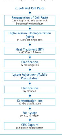
Figure 1. Primary recovery process scheme. Illustrates the sequence of unit operations required for the preparation of a Fab lysate feed stream suitable for the capture of Fab by cation exchange chromatography.
